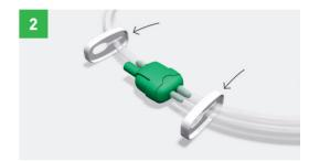
Clamp the canister tubing and dressing tubing by positioning the slide clamps next to the green connectors and slide across the tubings until secured.
