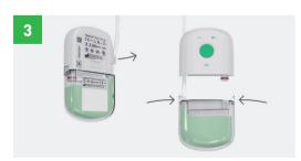
Release tubing at the back of the pump. Press hard on the side-mounted plastic tabs and pull while gently rocking to disconnect the canister. Connect the new canister. You should expect the canister to be a firm fit, this is normal and necessary for maintaining an effective seal.
